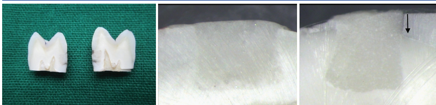
[Table/Fig-4]: Buccolingual section of the tooth. [Table/Fig-5]: Score 0-No marginal leakage. [Table/Fig-6]: Score 1-Less than and upto one half of the depth of the cavity preparation was penetrated by the dye. (Images left to right)
